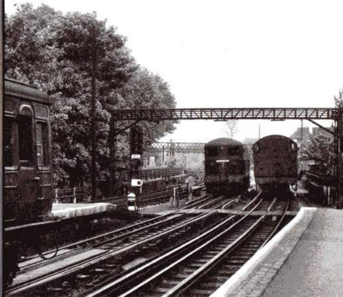
22 Locomotive changeover at Rickmansworth, May 1957. A train of compartment stock has been hauled from Aylesbury by a British Railways steam locomotive, moving away on the right, while Met electric loco number 7 approaches.
